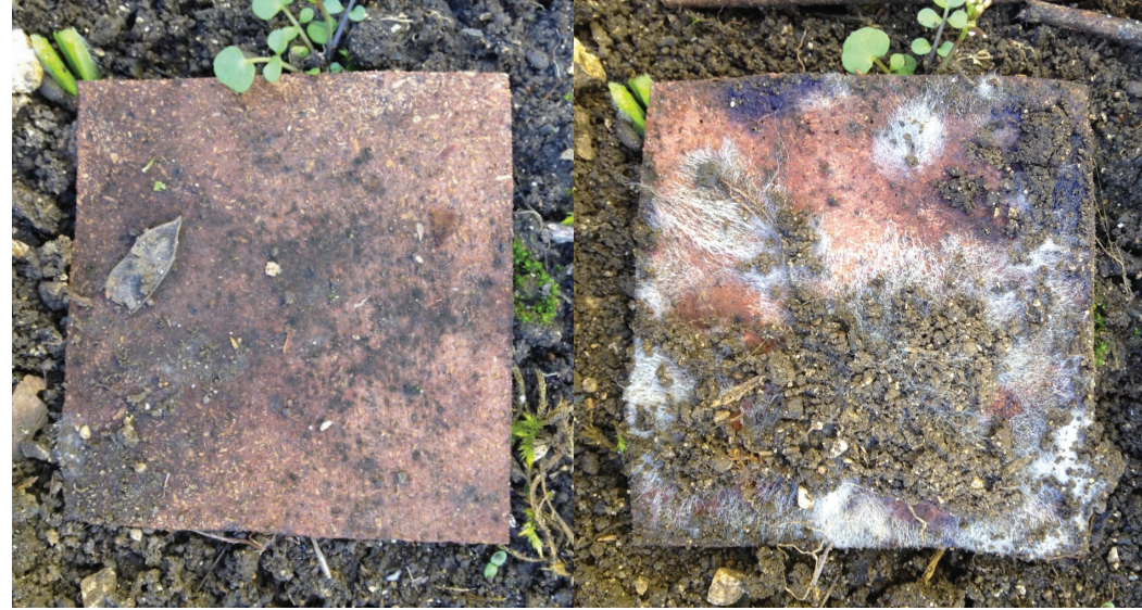
Test sample left outside, important degradation visible after 5 weeks (end of February/March 2016) Top/Under. © A.Q.
