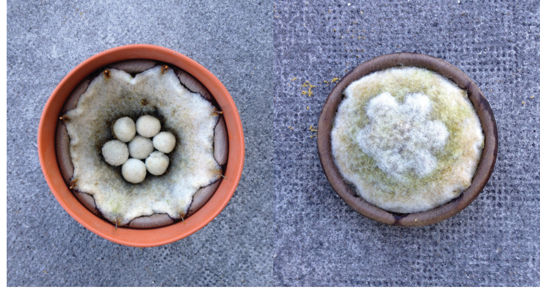
Shape which stimulates the degradation, left in an urban middle (Center of Lyon, results after 5 months). © A.Q.
