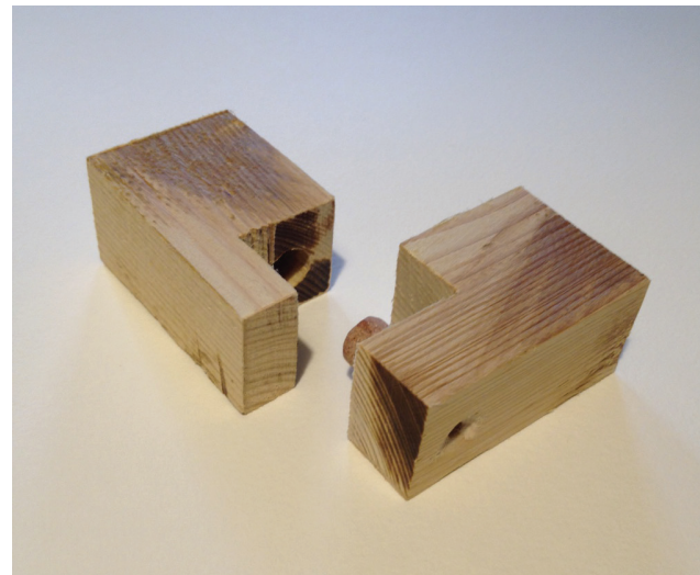
Dowels in assemblages shaped to degrade quickly with the rain © A.Q.
