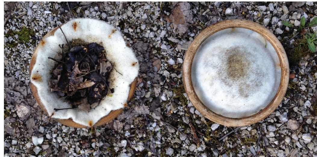
Shape which stimulates the degradation, left in a natural middle (Exposed to plants, results after 5 months). © A.Q.
