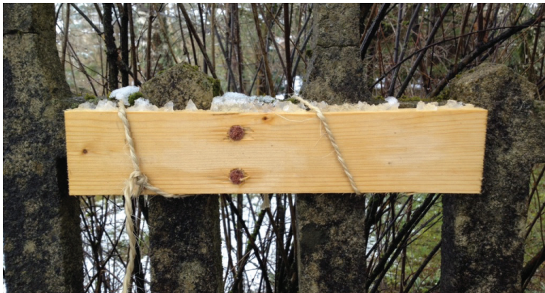
Test of assemblage with bioplastic dowels, reaction with the exterior conditions and the weight of the pieces of wood. © A.Q.
