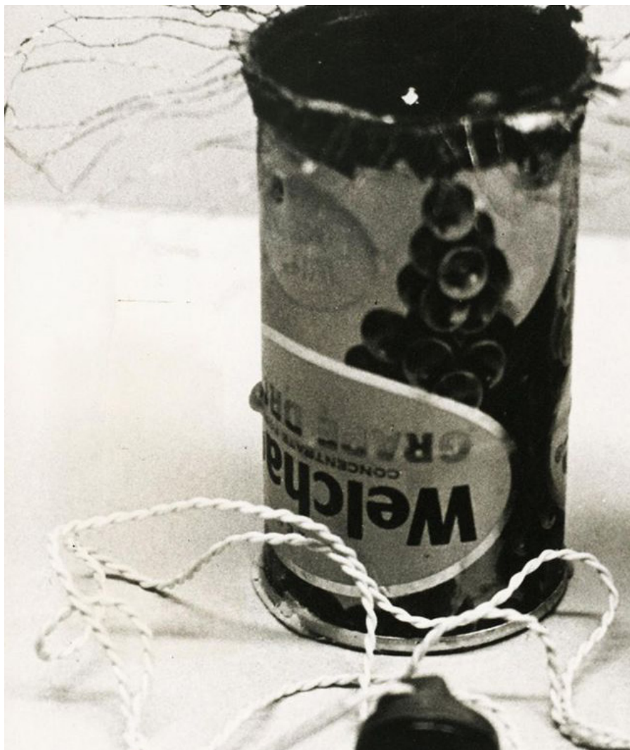
(fig. 13) Tin Can Radio, Victor Papanek and George Seeger, North Carolina State College © DR
